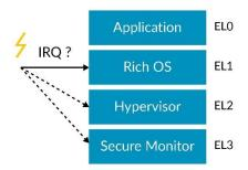
This routing is configured using SCR\_EL3 and HCR\_EL2. Routing configurations made using SCR\_EL3 will override routing configurations made using HCR\_EL2. These controls allow different interrupt types to be routed to different software.
