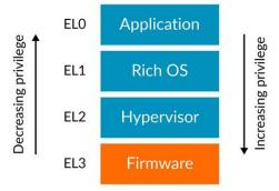
A common usage model has application code running at EL0, with an operating system running at EL1. EL2 is used by a hypervisor, with EL3 being reserved by low-level firmware and security code.
